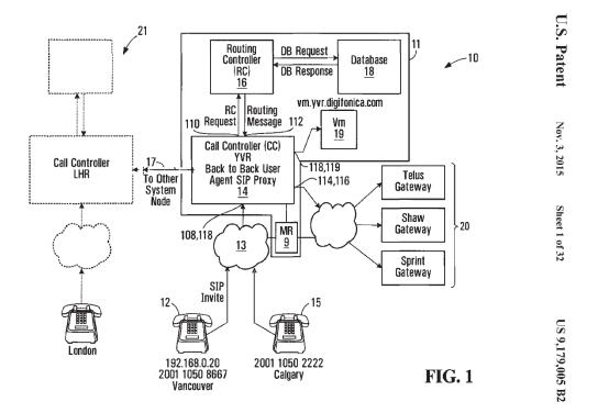
As is evident in Figure 1 above – that illustrates the environment of the invention required to make a phone call between London and Vancouver – the claimed inventions facilitate a phone call or other means of communication (12 and 15) within a multi-layered network whereby calls are routed by a physical controller (16) to physical gateways (20) and destination internet protocol addresses (12). APPX118,154 ('815 Patent)<sup>1</sup>.
